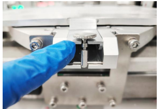
fig. 2-23 Rotate nut & insert into locking plate
