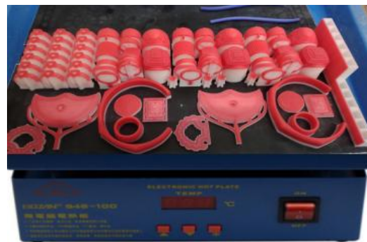
fig. 4-4 print build plate on hot plate
