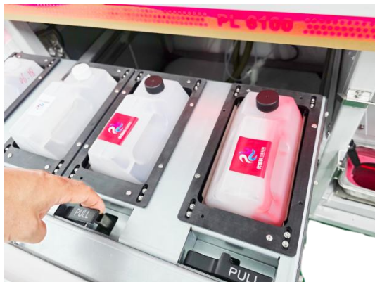
fig. 2-16 Material cartridge handle
