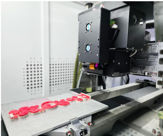
fig. 3-19 Print Build Plate stop position after printing
