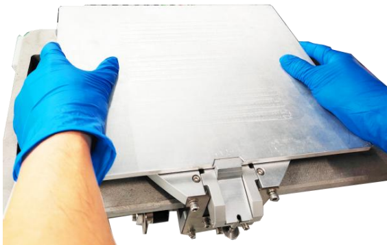
fig. 2-22 Press-down locking tab
