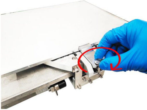
fig. 2-18 Turn the knob clockwise to loosen
