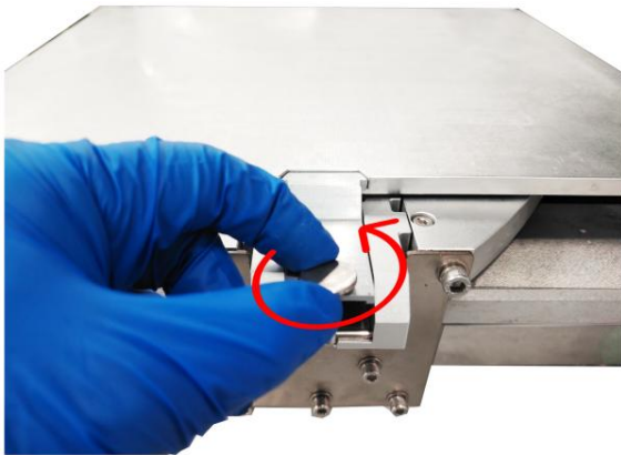
fig. 2-24 Rotate the locking nut anticlockwise.
